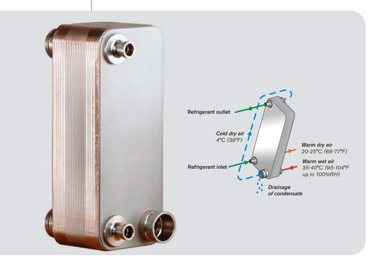
B12 Air-dryer combines cooling, condensing and heat recovery in one exchanger for high flow rates (12 Nm³/h). B12 Air-dryer combines extreme compactness with high heat transfer capacity in applications imposing high demands on dry, clean and conditioned air. The product is easy to customize, making it suitable for many different applications.
